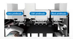
Extra printheads (factory option) can also be installed to handle MICR and other functional inks. With these optional heads, jobs that previously relied on overprinting can now be output in a single pass.
