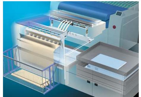
**3** The interleaf paper is lifted away and ejected into an external collection box.
