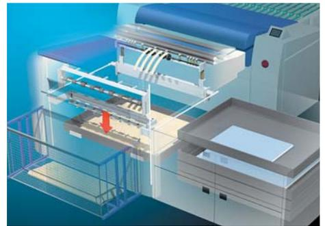
**2** The interleaf paper adheres to the suction pads and is removed.
