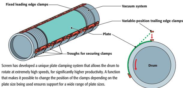
Screen has developed a unique plate clamping system that allows the drum to rotate at extremely high speeds, for significantly higher productivity. A function that makes it possible to change the position of the clamps depending on the plate size being used ensures support for a wide range of plate sizes.
