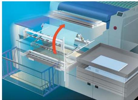
**1** The arm goes to pick up the plate, and the plate is hoisted up to the engine section.
