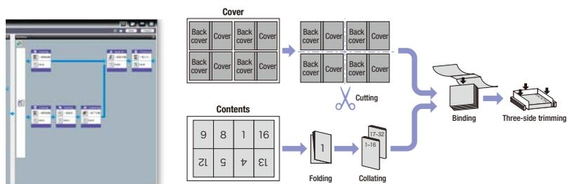
JDF data is automatically output to the post-processing equipment as soon as output of all signatures in a job finishes.
