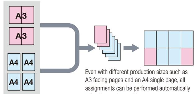
Even with different production sizes such as A3 facing pages and an A4 single page, all assignments can be performed automatically using the center position.
